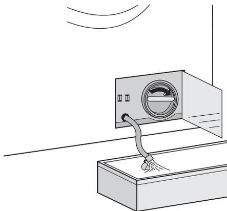
6. When no more water comes out, unscrew the pump and remove it. Always keep a rag nearby to dry up spillage of water when removing the pump.
