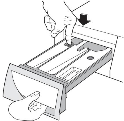
2. Remove the conditioner insert from the middle compartment.
