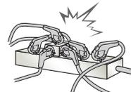
Do not plug too many electrical devices into a single multiple electrical outlet. Otherwise, this may result in fire due to over-heating.
