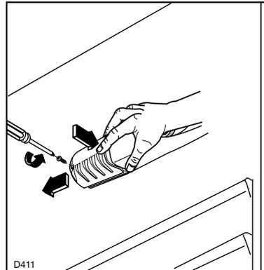
Unscrew the light cover and then pull it outward by pressing as shown in the figure. Unscrew the bulb and replace it with one of the same power (the maximum power is shown on the light diffuser) available from your nearest Service Force Centre.
