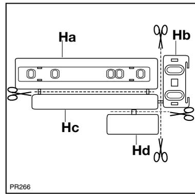
Place guide (Ha) on the inside part of the furniture door, up and down as shown in the figure and mark the position of external holes. After having drilled holes, fix the guide with the screws supplied.
