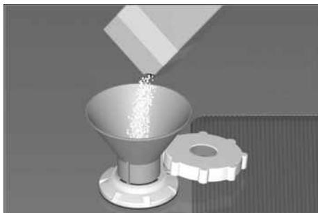
The LOW SALT indicator [6] on the front panel will light up initially but will extinguish again after a short period when the salt solution has become sufficiently concentrated.
